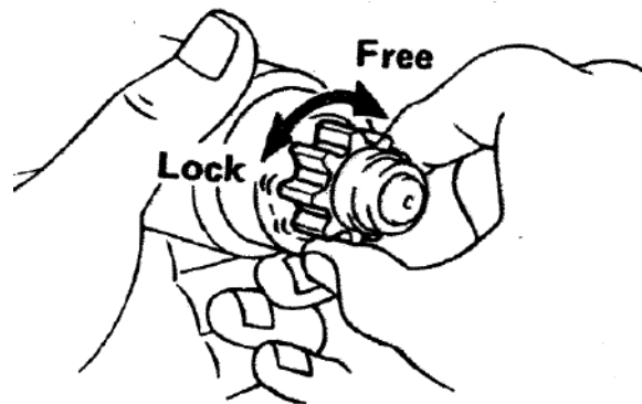
Gambar 2.71. Memeriksa pinion gear dan over running clutch
