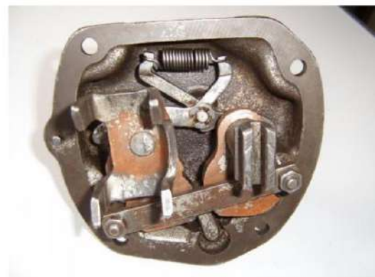
Gb. 2. Mekanisme double meshing prevention
