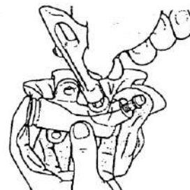
Gb. 17. Release silinder dan release fork
