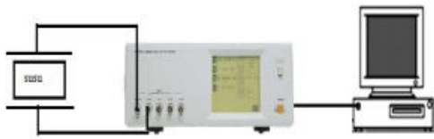
Figure 1. Measurement schema of cow's milk electrical properties with LCR meter
