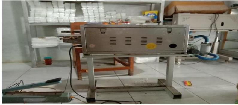
Gambar 1. 38. Mesin *Continuous Band Sealer* Fr900
