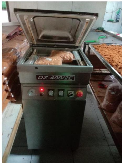
Gambar 1. 36. Mesin *Vacuum Packaging Dz-400/2e Standing Floor*
