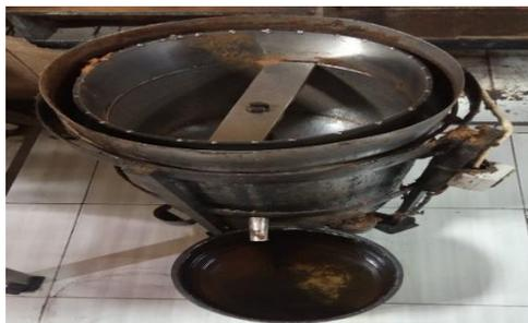
Gambar 1. 34. Mesin *Spinner Oil*
