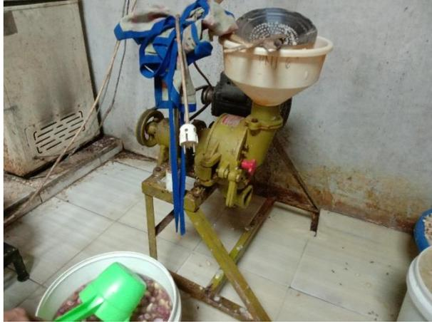
Gambar 1. 33. Mesin Pengupas Kulit Ari Kacang Bersistem *Rotary*
