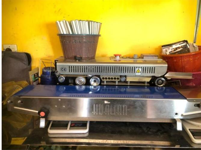
Gambar 3.1 Mesin *Press Pengemas Continuous Band Sealer*
