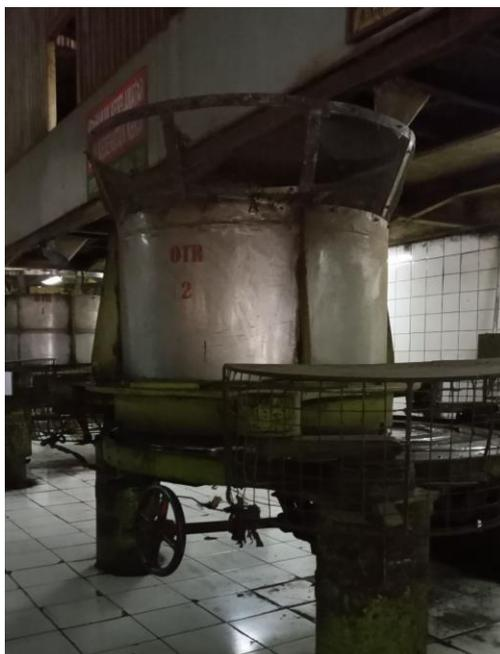
Gambar 1. 21 Mesin *Open Top Roller* (OTR)
