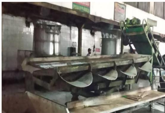
Gambar 1. 24 Mesin *Rotary Roll Breaker* (RRB)
