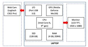
Fig. 4. Hardware design architecture
