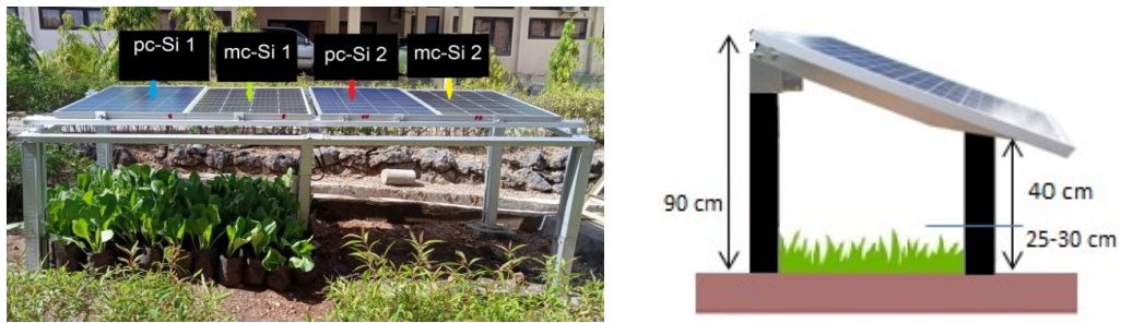
Fig. 4. Reference (pc-Si 1 and mc-Si 1) and vegetated (pc-Si 2 and mc-Si 2) PV modules
