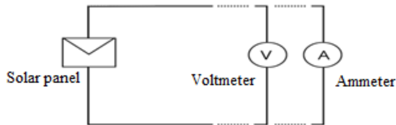
Fig. 2. Circuit diagram to measure I_{sc} and V_{oc} parameters
