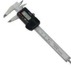
Gambar 5. Sliding caliper
