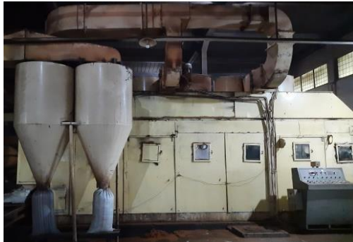
Gambar 1. 21. Fluid Bed Drier (FBD)
