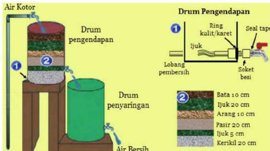
Gambar 4. Susunan Alat (Drum) Penjernihan Air Sederhana
