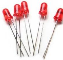
Gambar 2.15 LED (*Light Emitting Diode*)
