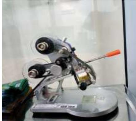
Gambar 1. 34 Mesin *Hot Code Printer* Getra DY-8B
