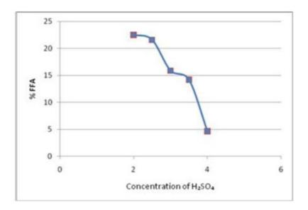
Figure 1. Graph of the relationship between the concentration of H<sub>2</sub>SO<sub>4</sub> and % FFA
