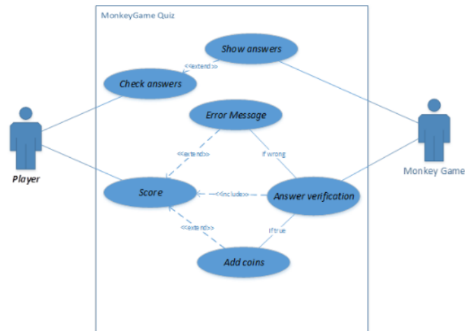
(b) Part Diagram of Main Use Case Containing Checking Answers and Feedback Figure 2. Digital Game Use Case Diagram
