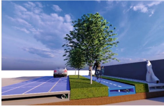
Fig. 2 A 3D simulation of prefabricated plastic panel utilization in the cycle and main roadway lanes
