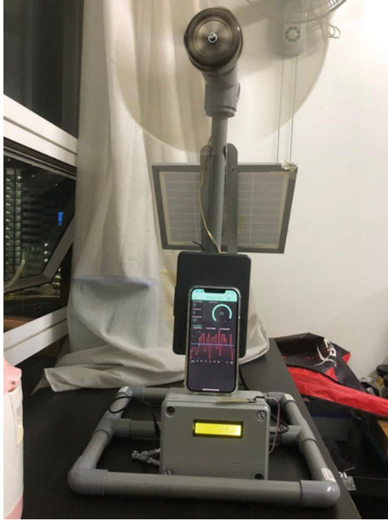
Fig. 3 The hybrid solar-wind system
