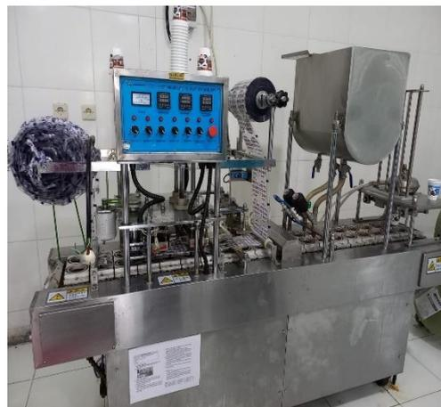
Gambar 1. 35 Mesin Automatic Filling Cup
