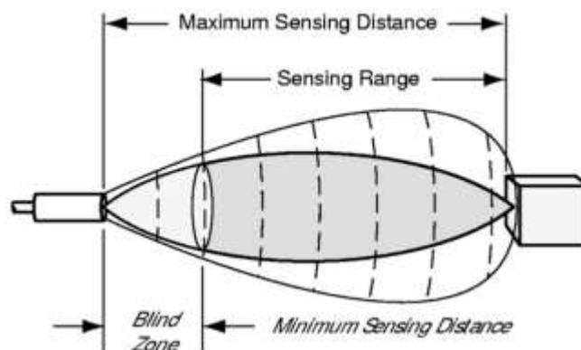
Gambar 2 Sudut pantul sensor Ultrasonik HC-SR04 [17]
