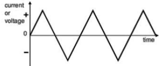
This triangular signal is AC because it changes between positive (+) and negative (-).
