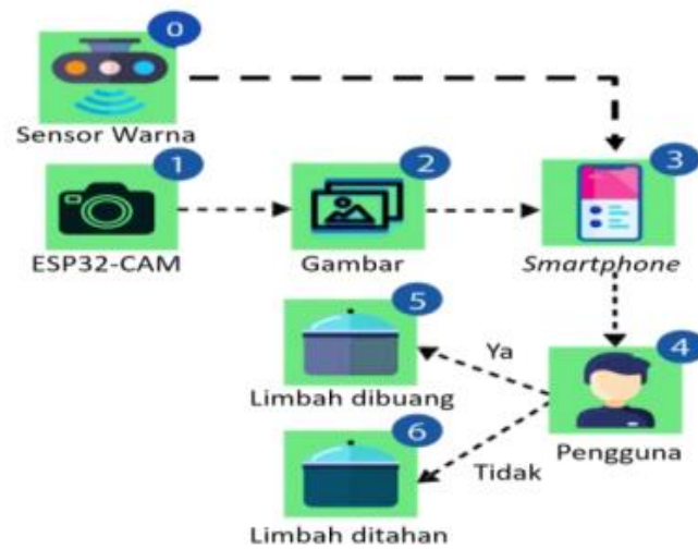
Figure 2. Working Principle of Batik Waste Processing Equipment
