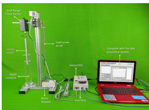
Figure 7. Image of the experimental apparatus based on Archimedes' principle for remote laboratory.
