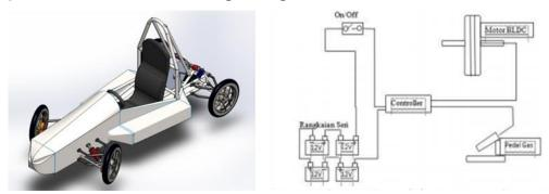
Figure 1. The Electrical Design of the AL-QORNI Electric Car
