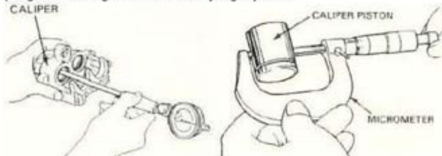
Gambar 36. Memeriksa Cylinder Caliper & Piston Caliper
