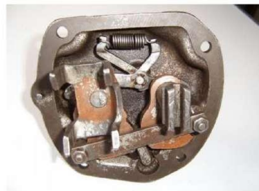
Gb. 2. Mekanisme double meshing prevention
