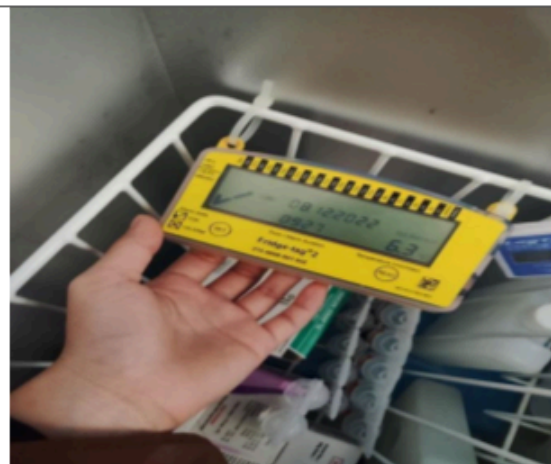
Figure 36. Fridge-tag used for maintaining the temperature of the vaccine storage in Yogyakarta
