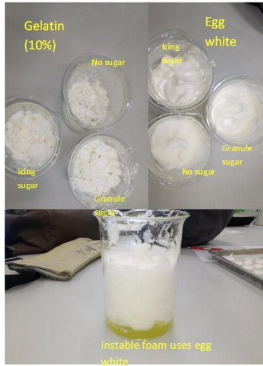
Figure 4. The photograph of foam formation from different emulsifier (upper), The instability of foam from egg white
