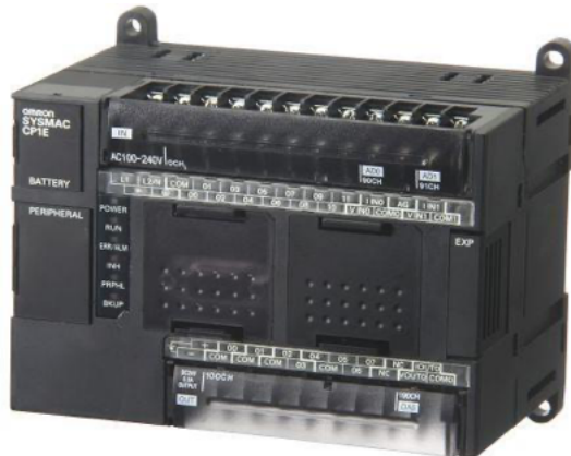
Gambar 1.2 PLC OMRON tipe CP1E NA20DR A
