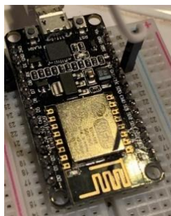
Figure 2. NodeMCU for designing IoT
