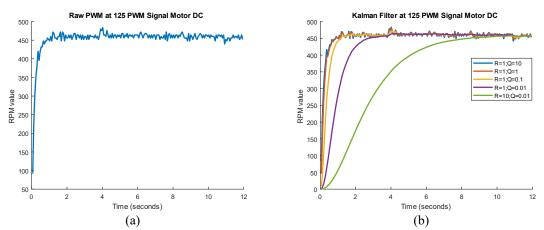
Fig. 5. Graph of tuning parameter Kalman Filter on speed Motor DC (a) Raw Data, (b) Filtered Data
