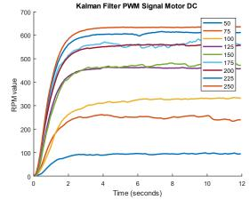
**Fig. 6.** PWM testing on Motor DC after Filtered with Kalman Filter (R = 1 and Q = 0.01).
