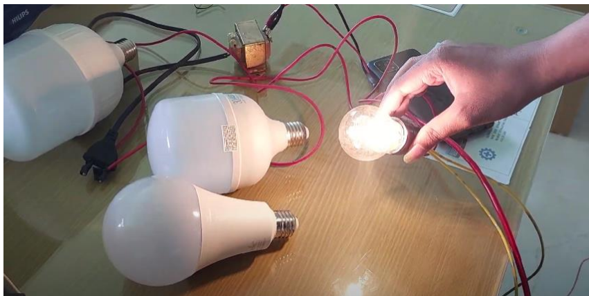
Figure 2. Inverter testing using a 5-watt load
