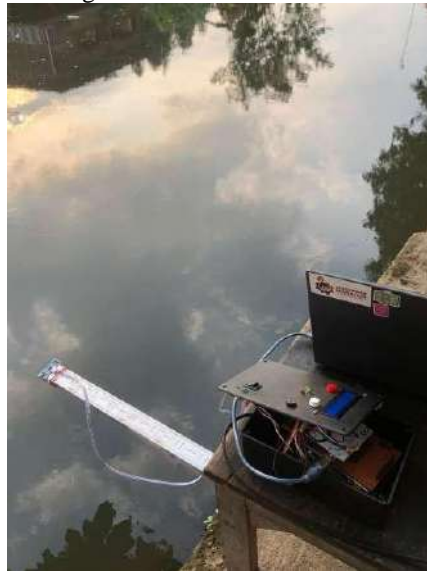
Figure 6. Ultrasonic Sensor Testing
