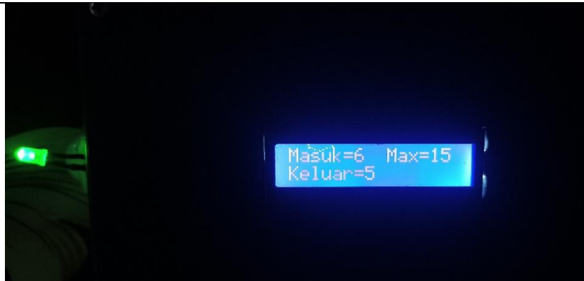
Figure 8. The exit LED is on
