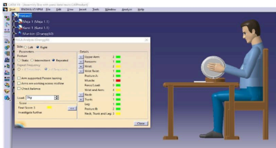
Figure 10 Posture analysis by RULA when operators do their jobs and viewed from right side
