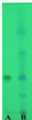
Figure 1. Thin layer chromatography analysis of quercetin standard (A) vs EERBL (B) with identical RF values, suggesting the presence of flavonoid quercetin in the EERBL
