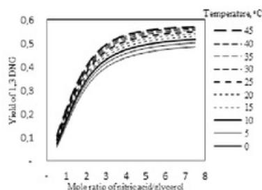
Fig. 4 Effect of mol ratio of nitric acid/glycerol to conversion of 1,3 DNG at concentration of HNO<sub>3</sub> 71.35% at various temperature
