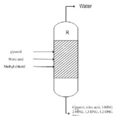
Fig. 2 Gibbs reactor (R) with specify equilibrium reactions type which was used for simulation
