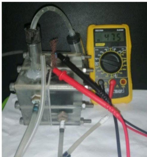
Figure 2. Photograph of MFC Setup and Operations Connected with a Multimeter Digital
