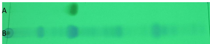
Figure 1. Thin layer chromatography analysis of quercetin standard (A) vs extract sample (B) with identical Rf values, suggesting the presence of flavonoid quercetin in the ethanolic extract
