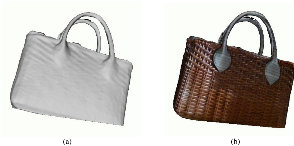
FIGURE 2. Scanning results: (a) colored vertices, (b) with raster surface
