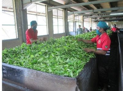
Gambar 1.13 *Withering Trough* (WT)
