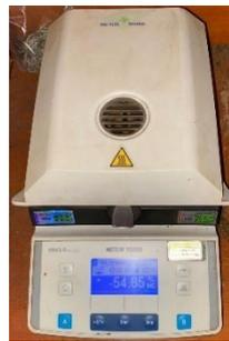
Gambar 2.1 Alat HB43-S Halogen *Moisture Analyzer*
