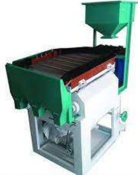
Gambar 1. 26 *Specific Gravity Sevarator (SGS)*
