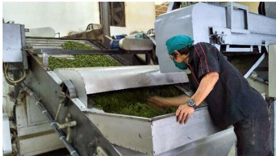
Gambar 1.19 *Endless Chain Pressure* (ECP)
