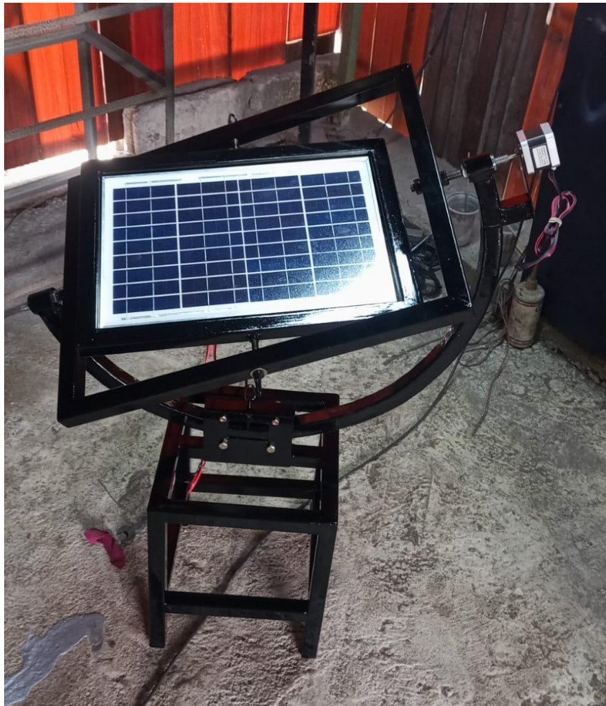
Gambar 9. Prototipe solar tracker
