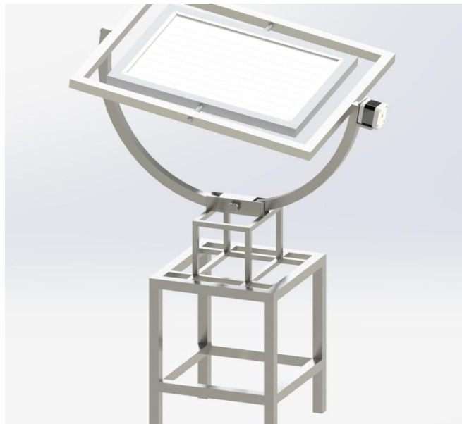
Gambar 7. Desain 3D solar tracker
