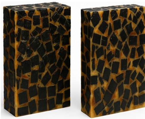
Figure 5. Marine Fender prototypes of waste tire and HDPE composites
